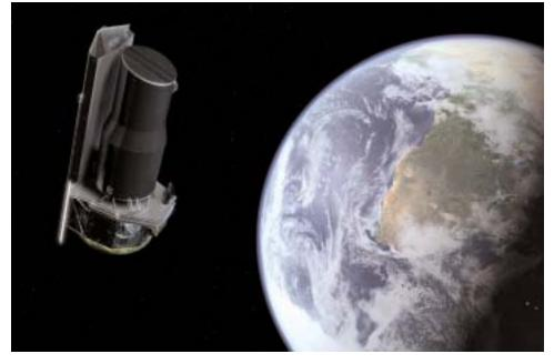
SIRTF - the Space Infrared Telescope Facility - was launched into space by a Delta rocket from Cape Canaveral, Florida on 25 August 2003. During its 2.5-year mission, SIRTF will obtain images and spectra by detecting the infrared energy, or heat, radiated by objects in space. Most of this infrared radiation is blocked by the Earth's atmosphere and cannot be observed from the ground.]
